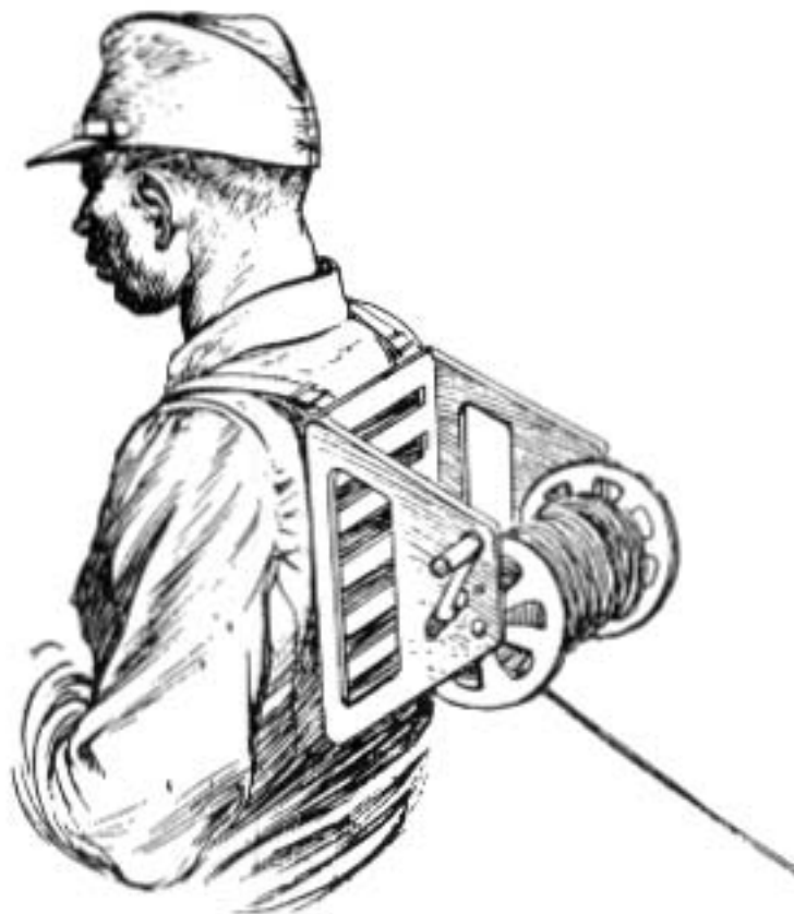
Figure 372. Head wire reel—used by field artillery. At left: Recovering wire. At right: Reeling out wire.
