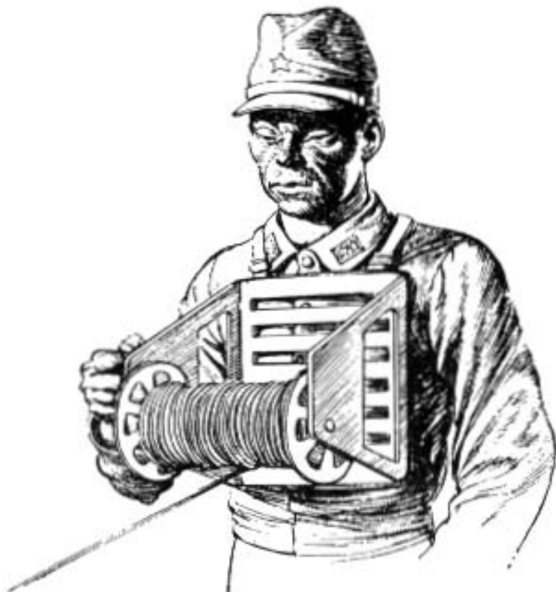
Figure 372. Head wire reel—used by field artillery. At left: Recovering wire. At right: Reeling out wire.
