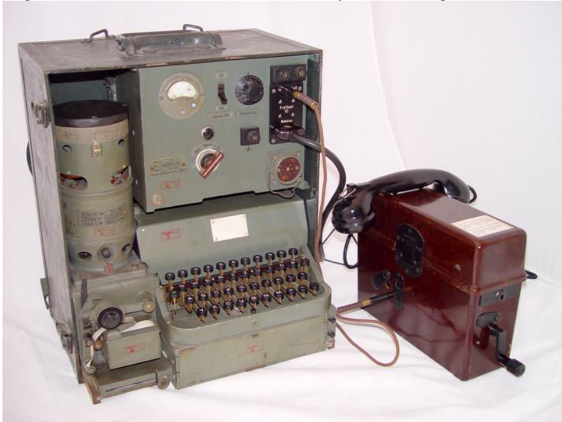
Figure 93: Feldfernschreiber plugged into an existing field telephone line
