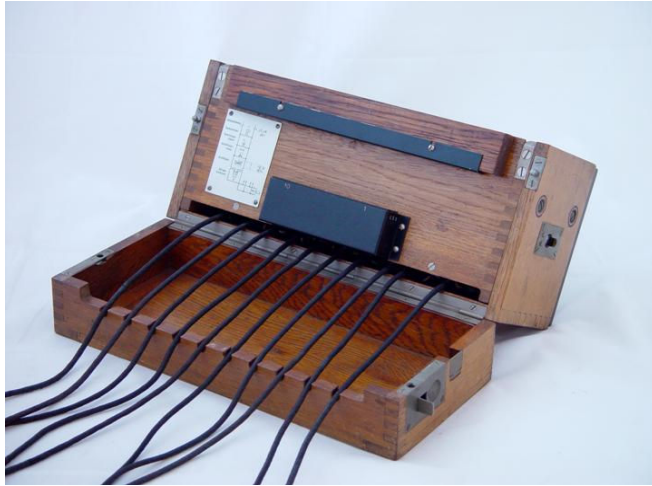
Figure 132: Klappenschrank cable storage compartment
