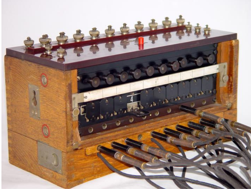
Figure 134: Klappenschrank incoming call on line 4, connected to line 8
