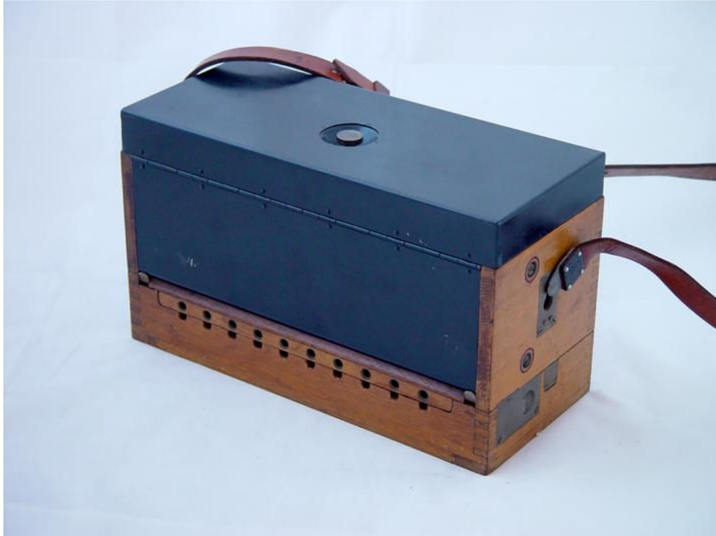
Figure 126: 10 line exchange in transport configuration
