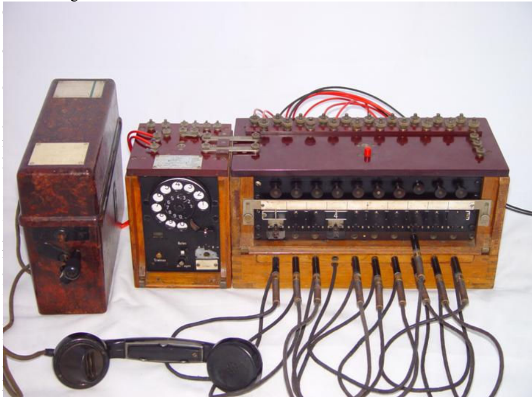
Figure 133: Klappenschrank ready for operation
