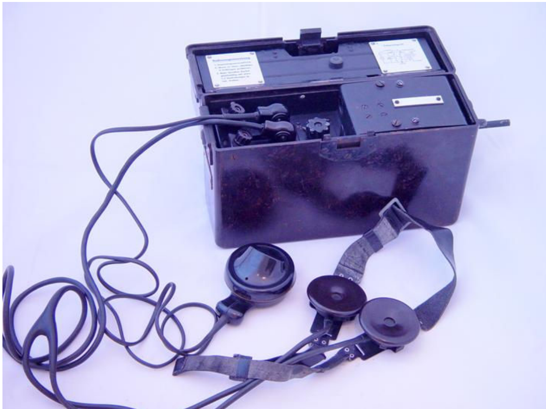
Figure 58: Erdsprechgerät with generator crank, headset and microphone connected
