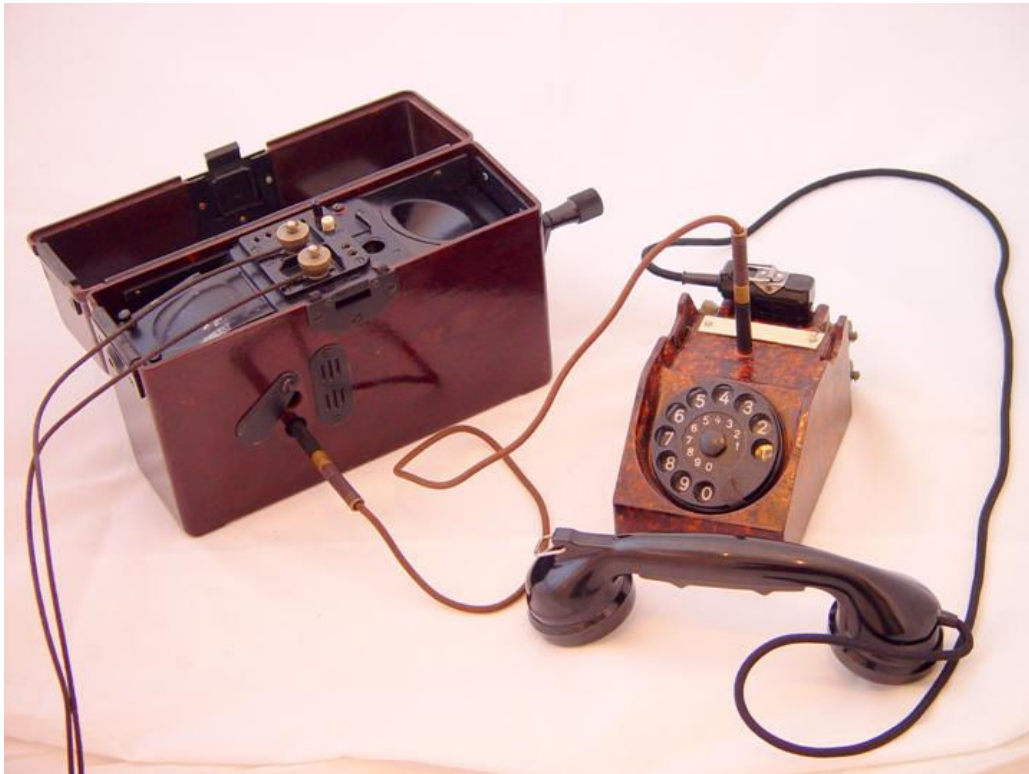
Figure 42: Amtsanschliesser connected to FF 33
