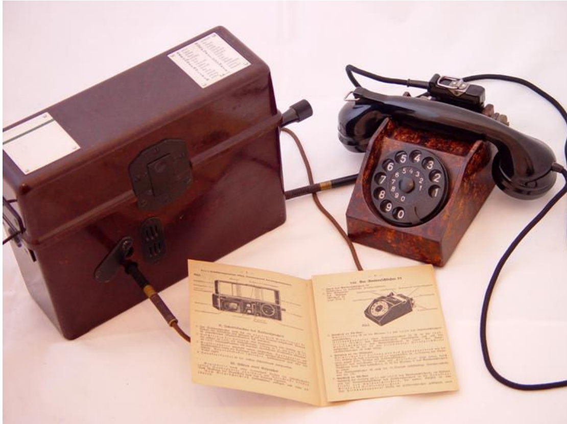
Figure 41: Amtsanschliesser 44 ready for use. Note instruction leaflet in front
